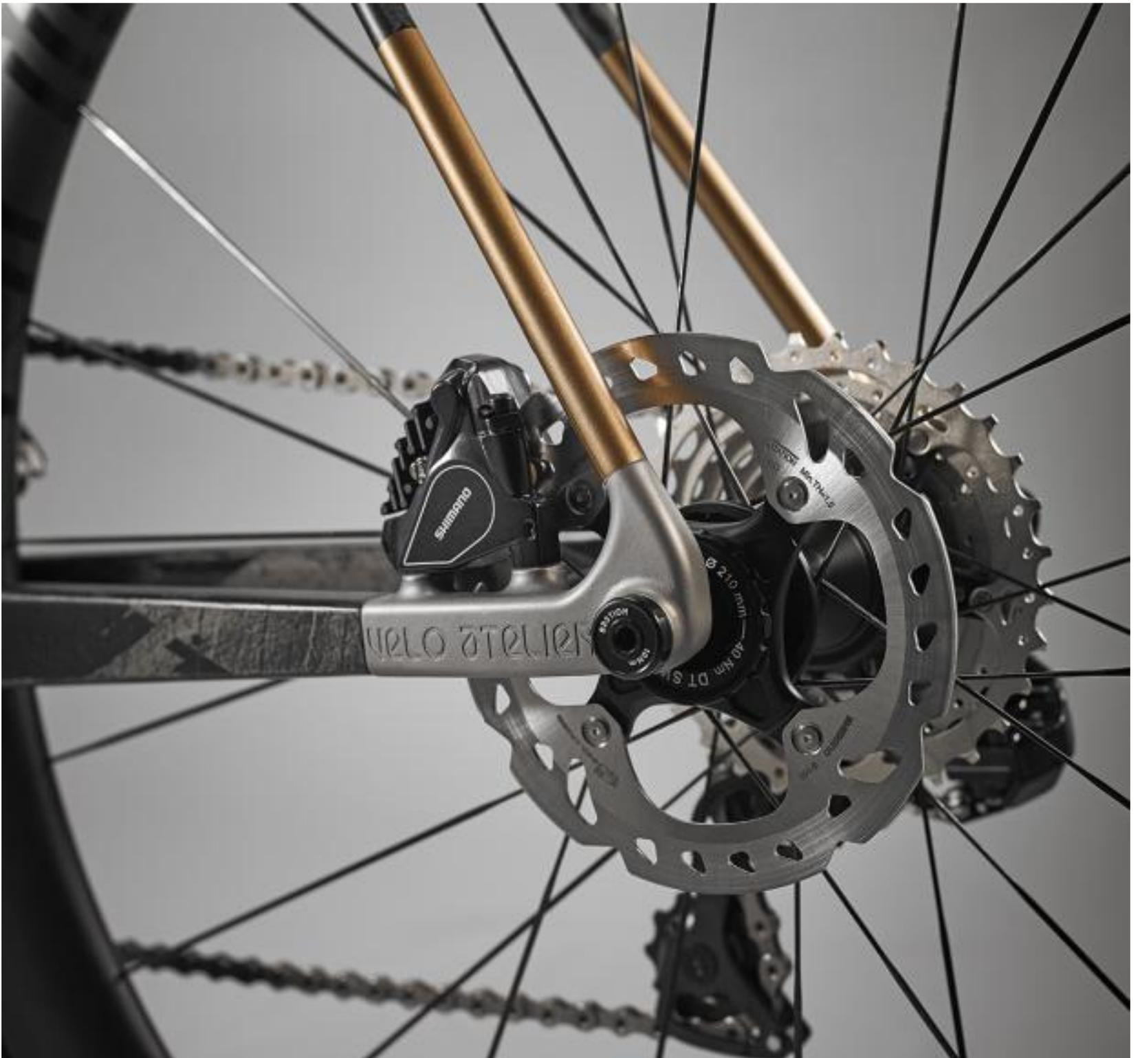
Holding the tubes together is the showpiece of the Bastion brand, thanks to the unique 3D printed titanium lugs (see The Detail box over the page).
